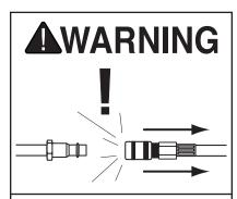
Always disconnect the air hose from tools whenever not in use or while servicing! During maintenance, a tool connected to air may operate accidentally, causing serious personal injury!
